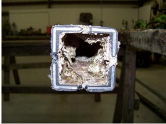
This cross-section shows the accumulation of marine life inside the post. The coating was not penetrated or damaged by the barnacles and other crustaceans.
